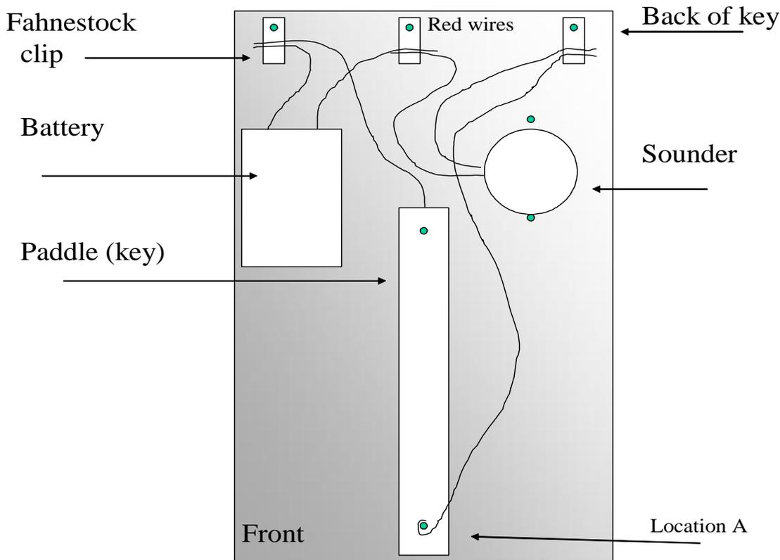
1. Red wires from battery clip and sounder unit attach to middle clip.
