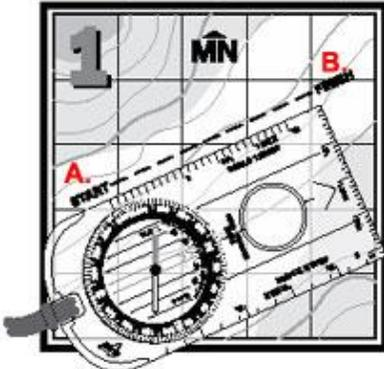
On the map align either the left or the right edge of the base plate through landmarks A and B with the direction of travel arrow pointing toward B.
