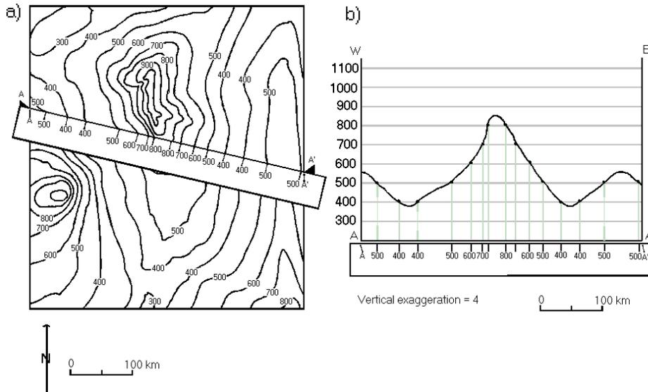
Figure 3. Illustration of how to draw a topographic profile from a contour map
