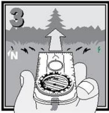
Read the bearing at the compasses index line, and follow the bearing in the field.
