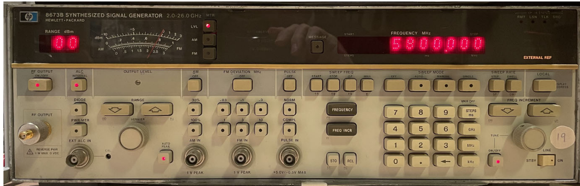
Fig 8 Synthesized Signal Generator HP 8673B (LO for HP 8971B, all instruments controlled by GPIB by the HP 8970B's system controller).
