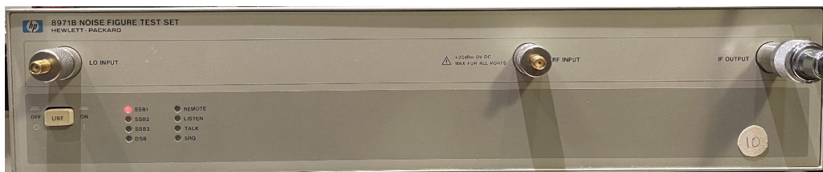
Fig 7 Noise Figure Test Set HP 8971B (part of the Noise Measurement System HP 8970S). At the LO input the HP 8673B is to be connected, at the IF output the HP 8970B respectively.
