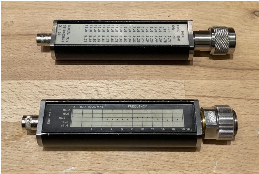
Fig 1 ENR-Noise Sources, HP 436A (upper), HP 436B (lower), each with calibration data.
