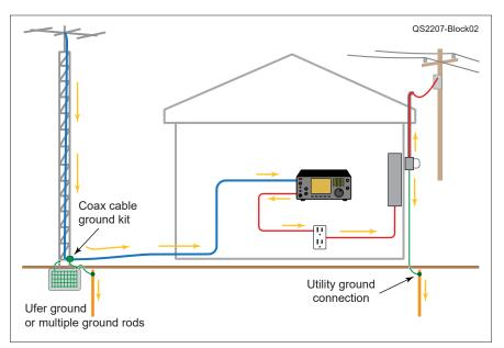
**Figure 2** — A simple installation where the radio is bridged across two non-interconnected grounds. The antenna ground is on the left and the ac utility ground is on the right. The surge energy is represented by the yellow arrows.
