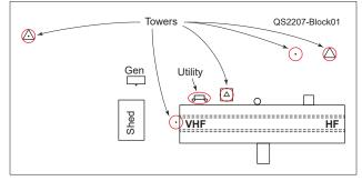
**Figure 1** — This drawing provides an aerial view of the clubhouse, showing non-interconnected earth grounds.
