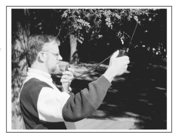
the antenna close to your head. Try to position the radio so the antenna is as far from your head (and especially your eyes) while transmitting. An external speaker microphone can be helpful.
