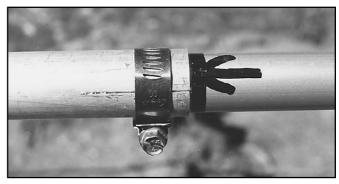
Figure 3—Use hose clamps to compress the slotted ends of the telescoping elements and keep everything in place. Marking the exact positions of the sliding tubes makes it much easier to assemble the antenna in the field.
