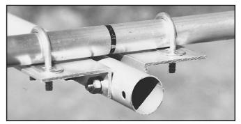
Figure 1—Two pieces of angle aluminum are attached to the boom with two nuts, bolts and lock washers. Your drilling must be accurate, so use a drill press if possible. In addition to drilling the boom holes, you'll need to drill four holes in each angle piece: two for accepting the boom-mounting nuts and two for the U bolts that will hold the element.
